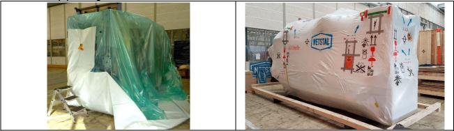
Machine is placed on steel-reinforced wooden bottom including fender, is wrapped in VCI preservative film and additionally will be shrink-wrapped in polyethylene film.
