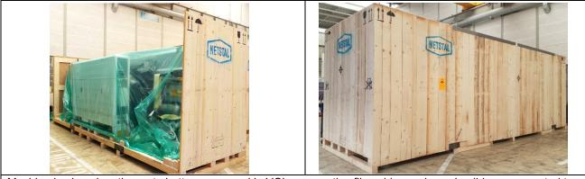
Machine is placed on the crate bottom, wrapped in VCI preservative film; sides and wooden lid are connected to each other.
