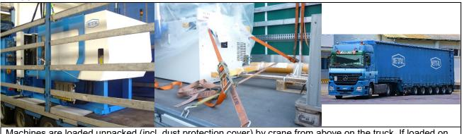
Machines are loaded unpacked (incl. dust protection cover) by crane from above on the truck. If loaded on an open loading platform due to oversize, a tarpaulin is needed to cover the machine completely!
