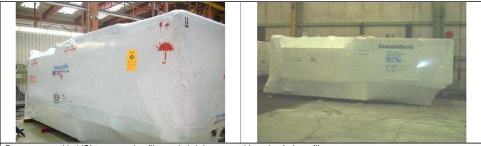
Parts wrapped in VCI preservative film and shrink-wrapped in polyethylene film.
