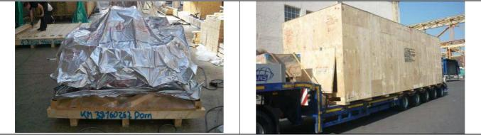
Parts are packed in barrier film (aluminium compound foil) with a desiccant and attached to the bottom; sides and wooden lid are connected to each other.
