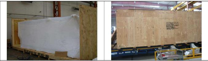
Parts wrapped in VCI preservative film, shrink-wrapped in polyethylene film and attached to the bottom; sides and wooden lid are connected to each other.
